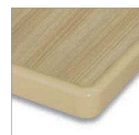
AP01-08 25 mm work surface 0.8 mm HPL coated oak, 8 mm PUR edge beige
